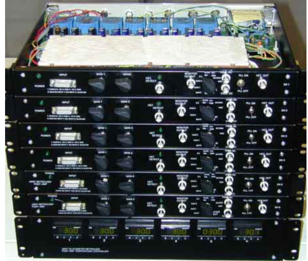
Fig 11. Photo of JWST/TPF metrology post-amps. Top module is open, showing multiple power supplies (rear) and the constant temperature oven (front). The bottom module is a six-channel temperature controller maintaining the ovens at 30.0 C.
